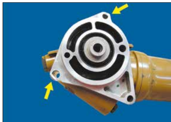
Figure 2 - no core refund Pump with non-operational damage
