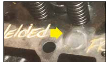
Figure 7 - damaged core refund This head had a top deck crack and was repaired by welding the freeze plug hole shut. Perkins does not use or authorise this process
