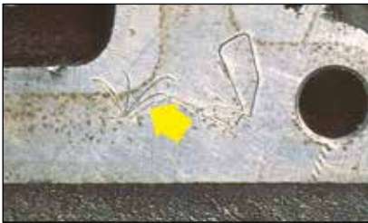
Figure 1 - damaged core refund Welder's mark
