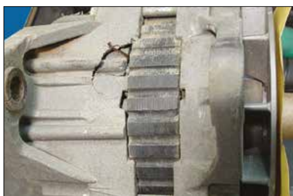
Figure 3 - damaged core refund Cracked housing
