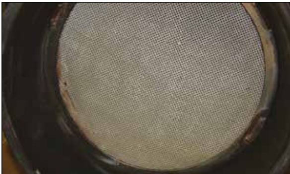
Figure 3 - damaged core refund Honeycomb chipping exceeding two radial cell limit
