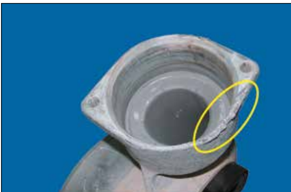
Figure 3 - full core refund Damage - chipped cold housing
