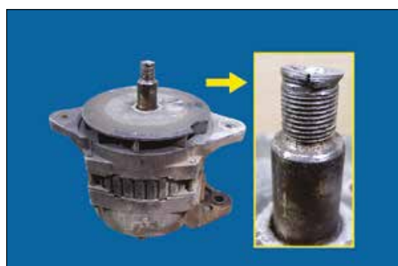
Figure 4 - damaged core refund Non operational damage - hammer strike to shaft
