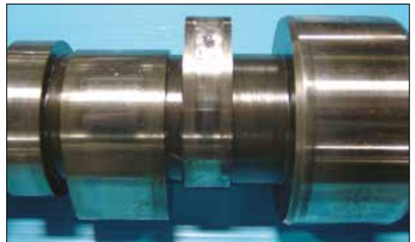
Figure 4 - full core refund Material missing on lobe
