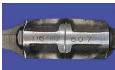
Figure 6 - full core refund Cap and rod markings matched
