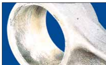
Figure 3 - no core refund Pin bore damage
