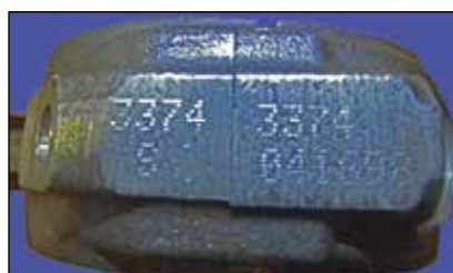
Figure 5 - full core refund Cap and rod markings matched
