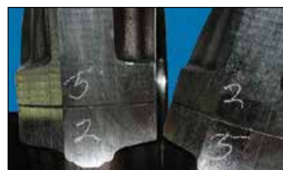
Figure 7 - no core refund Mismatched cap
