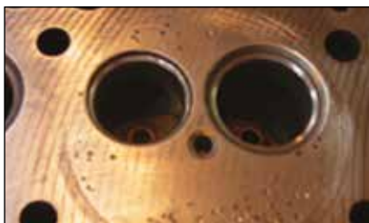
Figure 4 - damaged core refund Dropped valve damage
