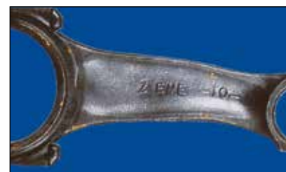
Figure 4 - no core refund Visibly bent and twisted
