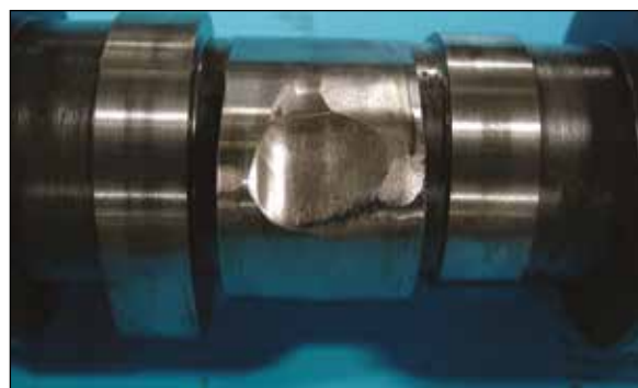
Figure 5 - full core refund Material missing on lobe
