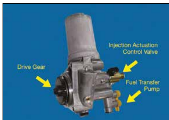
Figure 4 - full core refund Pump group complete with drive gear, injection actuation control valve and fuel transfer pump
