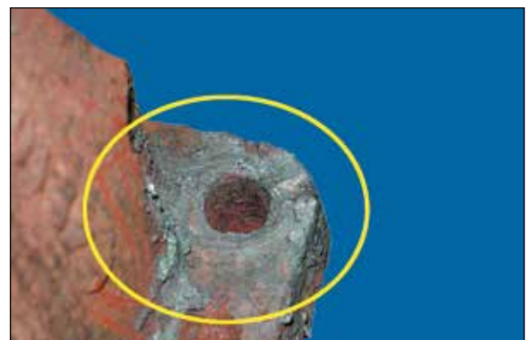
Figure 9 - damaged core refund Non-operational damage - melted by torch
