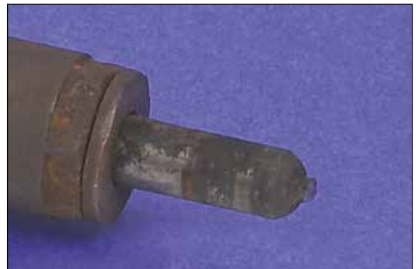
Figure 2 - full core refund Damaged nozzle
