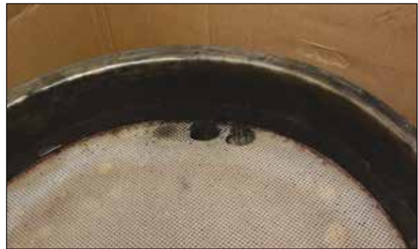
Figure 2 - damaged core refund Honeycomb cracking
