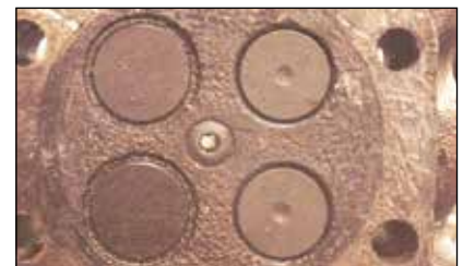
Figure 8 - full core refund Pitting
