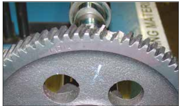
Figure 2 - full core refund Damaged gear
