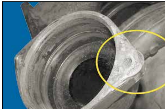
Figure 5 - full core refund Turbo with hammer marks/blows on cold housing
