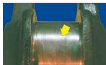
Figure 2 - no core refund Visible crack
