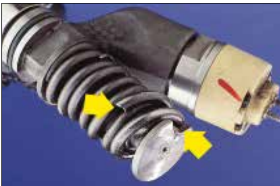
Figure 3 - full core refund Broken tappet and spring
