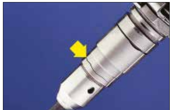
Figure 4 - no core refund Cracked body
