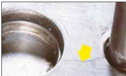
Figure 3 - damaged core refund Top deck crack
