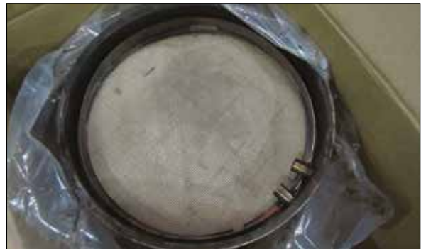
Figure 4 - damaged core refund Operational damage - indicates internal cracking that is passing soot
