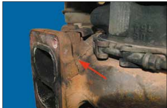
Figure 2 - full core refund Operational damage - crack
