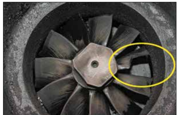
Figure 7 - damaged core refund Hot wheel broken
