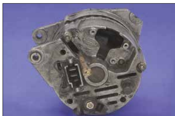
Figure 2 - damaged core refund Broken housing
